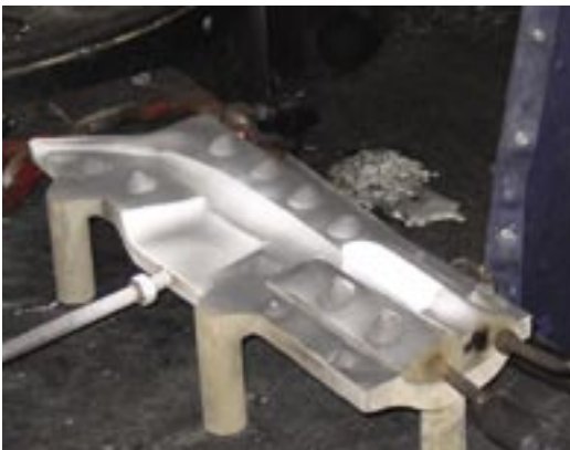
1. View of the bottom half of die, with die-blocks inserted. The feeder-point at the top can be seen, along with overflow cavity at side, and locating points on the face of the die.
