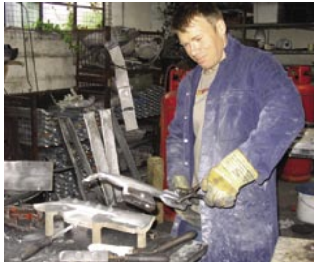
3. Removing the casting from the die, with the feeder sprue and overflow block attached.
